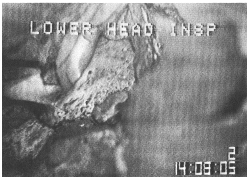
Figure 18. Former liquid material which appears to have dropped to the curved area of the reactor vessel lower head and flowed some distance.
