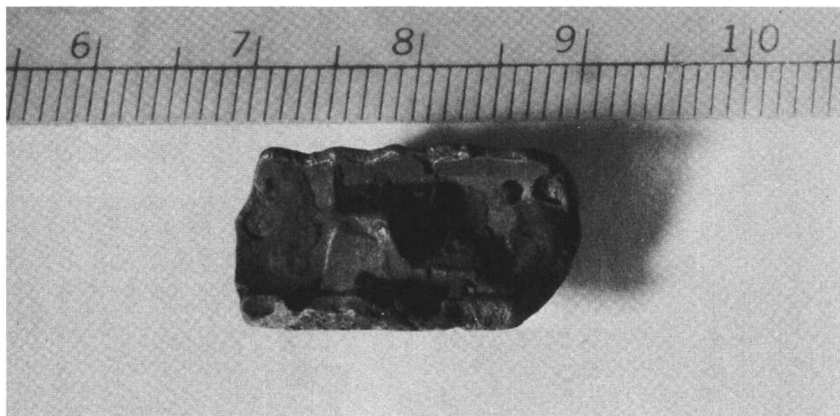
Figure 4. Fuel rod segment from surface of debris bed at H8 location (Sample 1A).
